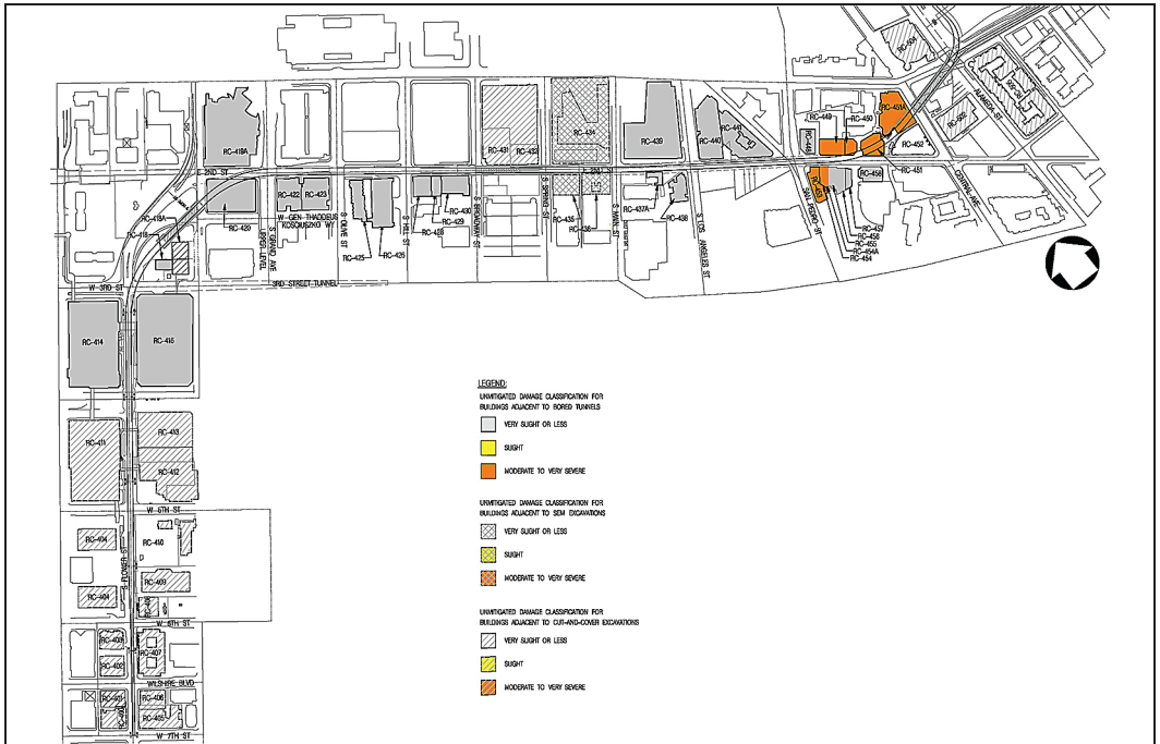
Figure 5. Adjacent buildings impacted by bored tunnels and cut-and-cover excavations
